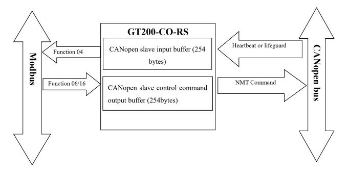
As is shown above, the gateway assigns 2-byte status input buffer and 2-byte control command output buffer (it can have up to 127 nodes in CANopen, so the aggregates is 254 bytes) for each CANopen slave respectively. So, Modbus master can use function 04 to read status of each CANopen slave and also can use function 06 or 16 to control the running state of CANopen slave.
