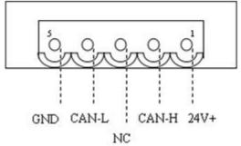
Note: Voltage between 24V+ and GND is 24V, power range is 11V~30V.
