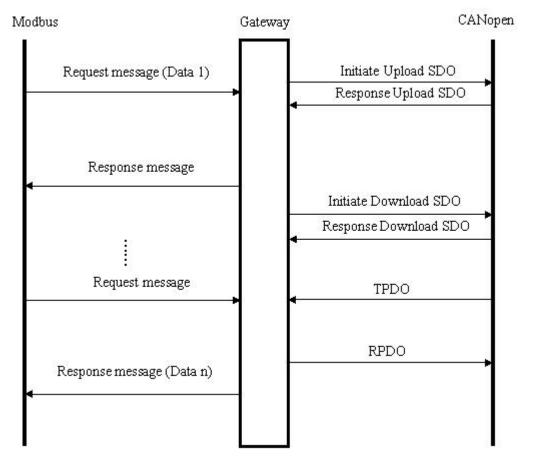
"Data 1" shows the data transfer process from Modbus to CANopen; "Data 2" shows the data transfer process from CANopen to Modbus.
