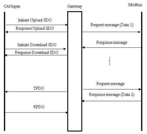
"Data 1" shows the data transfer process from CANopen to Modbus; "Data 2" shows the data transfer process
