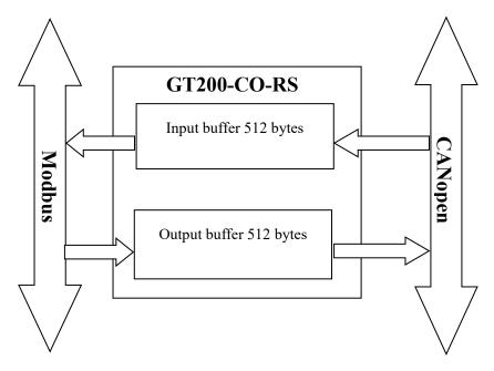
Modbus master reads 512 bytes input buffer data through No.4 function code, write data into 512 bytes output buffer through No.6&16 function code, and read 512 bytes output buffer data through No.3 function code. Input buffer address range: 0x0000~0x01FF;
