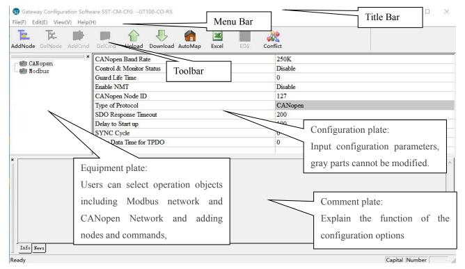
For detailed software content, please open the SST-CM-CFG, select "Help" >> "Content" on the menu bar.
