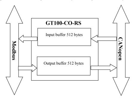
Modbus master reads 512 bytes input buffer data through No.4 function code, write data into 512 bytes output buffer through No.6&16 function code, and read 512 bytes output buffer data through No.3 function code.
