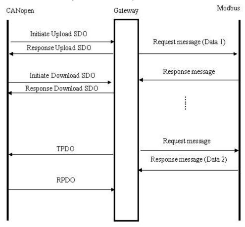
"Data 1" shows the data transfer process from CANopen to Modbus. "Data 2" shows the data transfer process from Modbus to CANopen.
