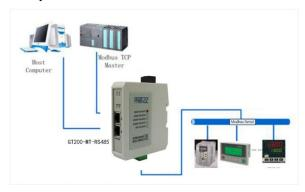
2. Multiple serial port master stations connect multiple Modbus TCP server stations
