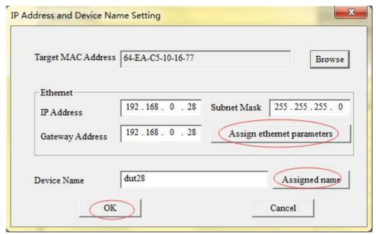
You can see that after log in the device "Target MAC address" shows MAC address of GT200-PN-RS (unmodified).
