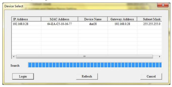
You can see that GT200-PN-RS device is on the LAN, showing its "IP", "MAC address", "Device Name", "Gateway" and "Subnet".
