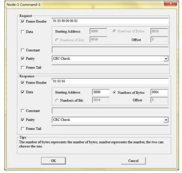
Notes: Under RTU transmission format, supports following parity: None, CRC check and sum check For example, configuring Modbus command, ASCII transmission format:
