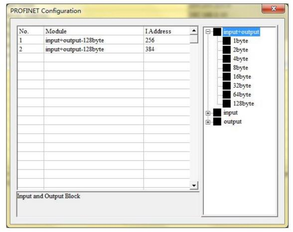
As is shown above, there are 2 slots configured, that is: 128byte input + output, 128byte input + output. The same as STEP7 module, users can drag the data module on the right side to the left slots.
