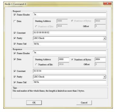
Notes: Under ASCII transmission format, supports parity: None, LRC check and sum check
