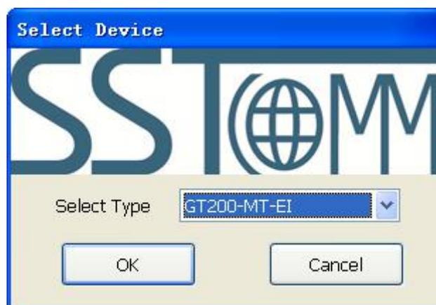
Select “GT200-MT-EI”, click OK to enter into the main interface of GT200-MT-EI (enter into the default parameters setting interface of EtherNet/IP. Click the Ethernet type of equipment view interface to switch the parameters setting interface.
