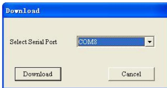
**Remark 1:** Please check the port in "COM Config" is the port that you are using before downloading the configurations;
