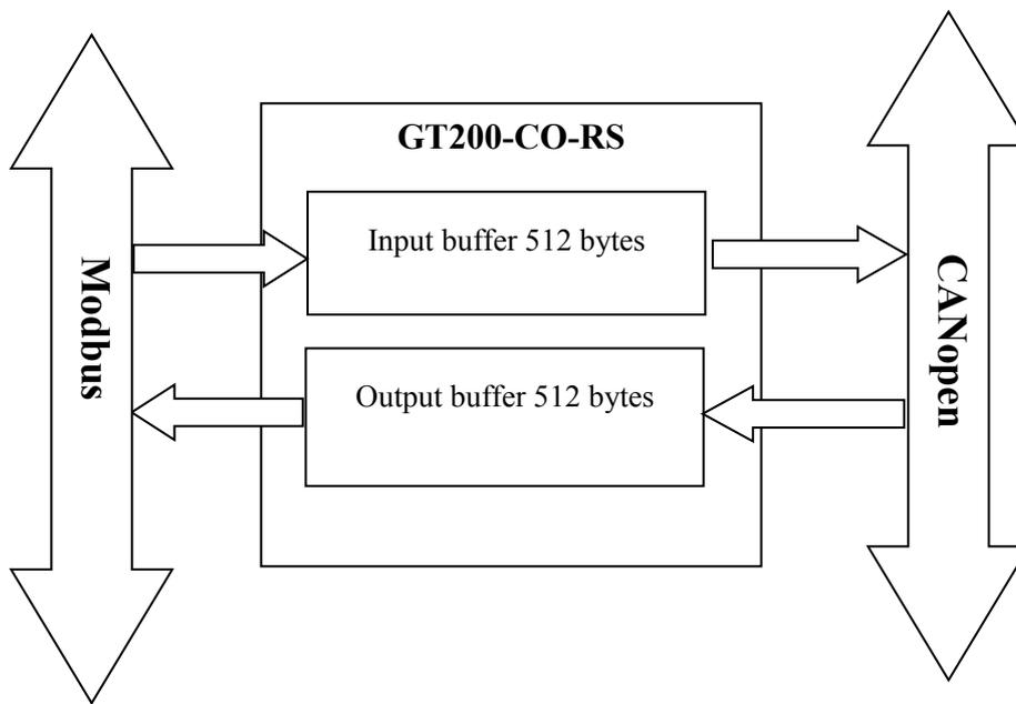
Input/output buffer supports fast SDO visit, the position where input/output buffer is located in the object dictionary is listed as below table:
