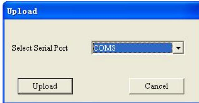
**Remark:** Please check the port in "COM Config" is the port that you are using before uploading the configurations;
