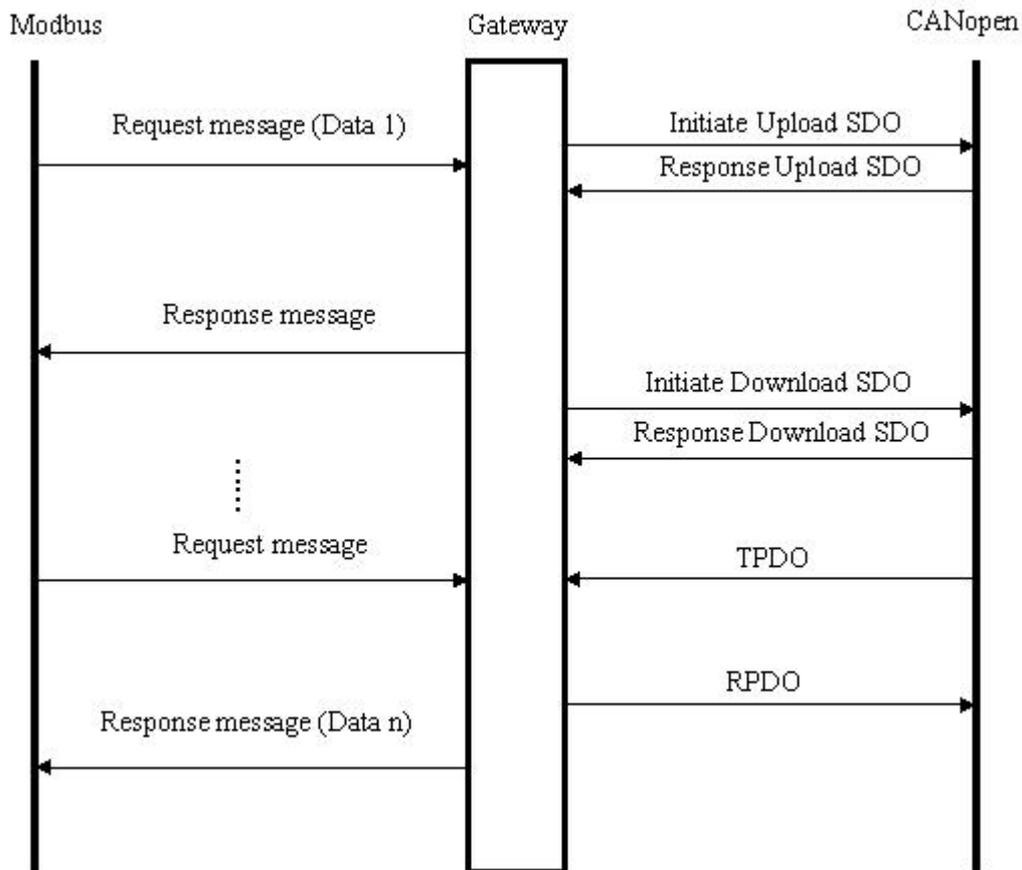
“Data 1” shows the data transfer process from Modbus to CANopen; “Data 2” shows the data transfer process from CANopen to PROFIBUS.
