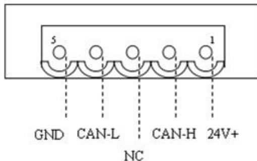
Note: Voltage between 24V+ and GND is 24V, power range is 11V~30V;
