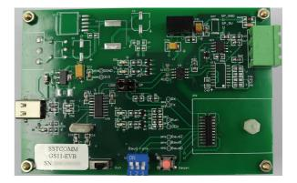
The EV board uses a three-pin pluggable terminal for RS-485, the description show as follow:
